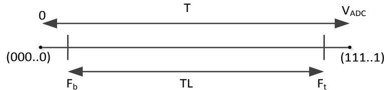
Figure 3.1: Figure showing the total range, T (Codes 000...0 to 111..1) and the linear input range, TL ( F_t to F_b ) of ADC. T = TL if, F_t = 111..1 and F_b = 000..0 .
